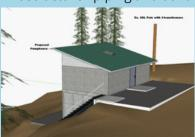
the project. The new pump facility building allows for a consolidation of control functions, water quality monitoring, and increased instrumentation. This project results in a major upgrade for the primary wellfield and distribution hub for the water district that will serve us well into the future. We expect to be completed in the Spring.
