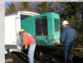
← 80kw Standby Generator loaded into trailer rig – this is so we can keep your water flowing during an extended power outage!
